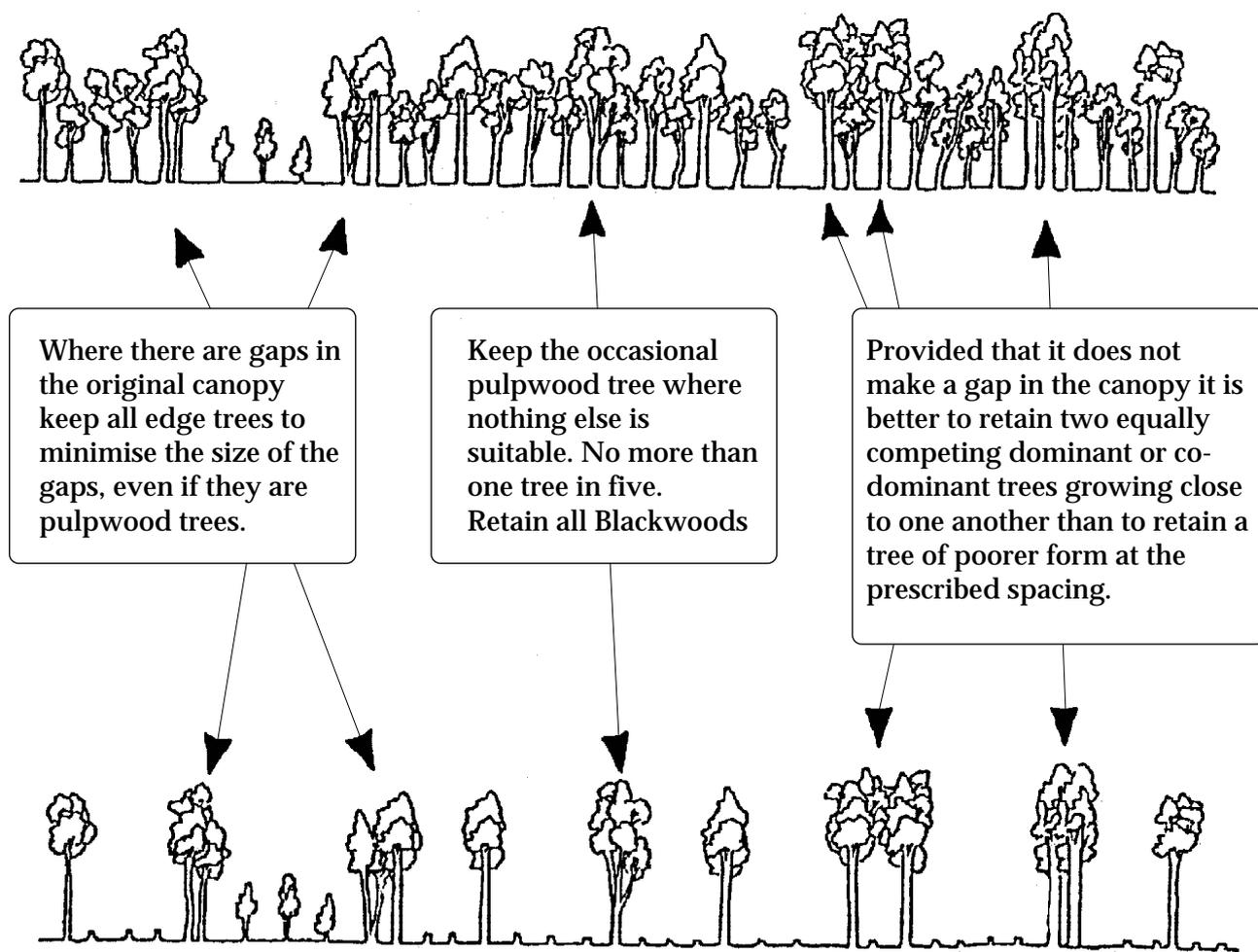
Figure 16. Some spacing guidelines to achieve an even retained canopy.
