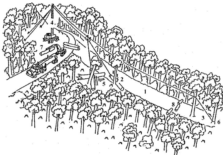
Figure 14. The damage minimisation precautions for a cable thinning operation.
