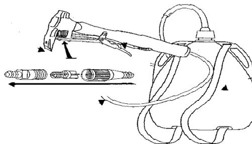
Figure 9. Stem injector unit
