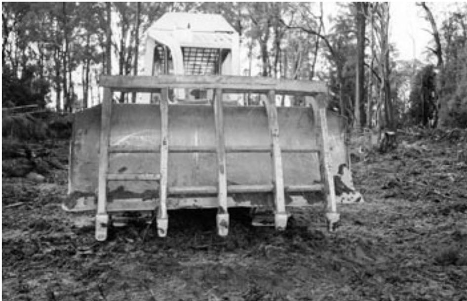
*Photo 3. Front-mounted root rake on the International TD15 bulldozer.*
