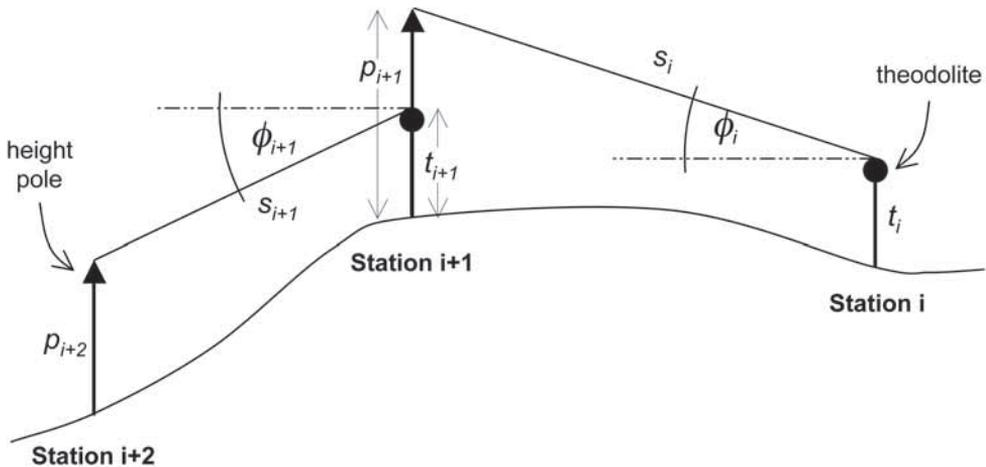
Figure A2.1. Notation for station traverse.
