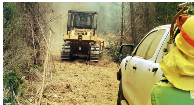
STTas firefighting vehicle monitoring the safety of bulldozer operator while cutting track along a fire perimeter.
