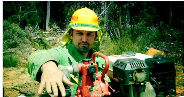
*STTas officer operating water pump to draw water from a water point (waterhole, dam, stream etc) into the water tanker.*
